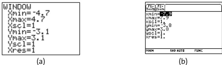
Figure 2.26 The Window editor screen on the (a) TI-83 and TI-84 (b) TI-89 Titanium.
